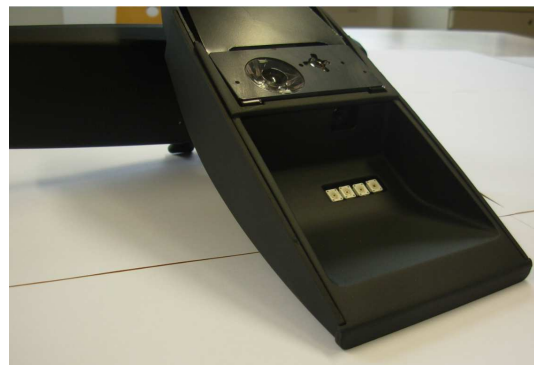
MFOS sensor prototype integrated in the internal rearview mirror
